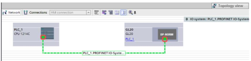
d. Double-click the GL20-RTU-PN module in the network view to open the device view, as shown in the figure below.
