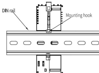
2. Make sure the DIN rail mounting hook of the module is locked. The locked and unlocked states of the mounting hook are shown below.
