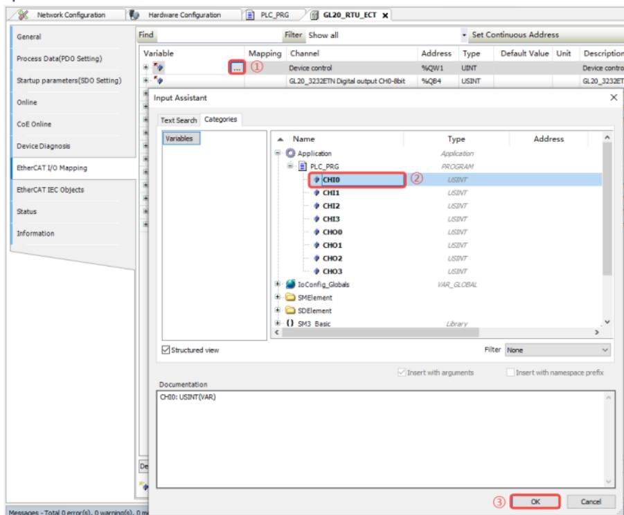
c. Map the input variables "CHI0", "CHI1", "CHI2", and "CHI3" to the input channels of the configuration module, and map the output variables "CHO0", "CHO1", "CHO2", and "CHO3" to the output channels of the configuration module, as shown below.
