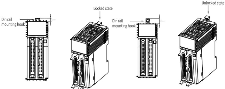
To lock the module to the DIN rail, press down the mounting hook.
