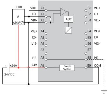
Three-wire voltage wiring
