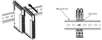
Make sure the DIN rail mounting hook of the module is locked. The locked and unlocked states of the mounting hook are shown below.
