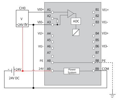
Four-wire current wiring
