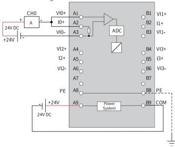
• Three-wire current wiring
