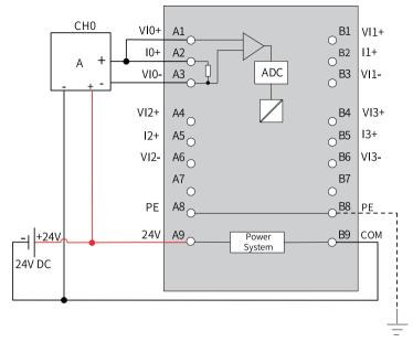
• Four-wire voltage wiring
