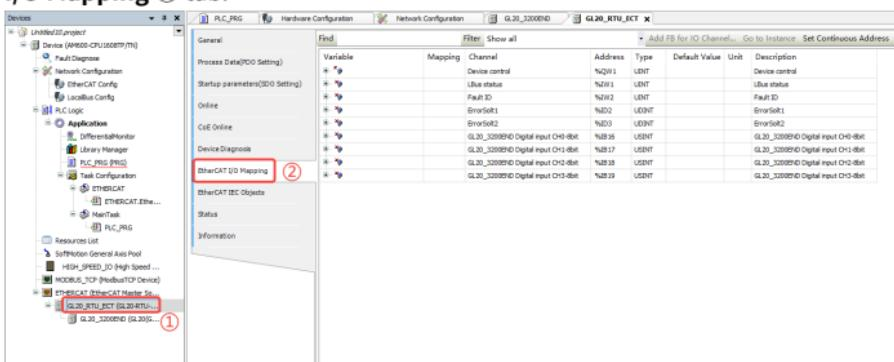
b. On the **EtherCAT I/O Mapping** tab, double-click a variable entry and click ① to open the **Input Assistant** dialog box. Choose **Application > PLC\_PRG >** specific variables ② and click **OK** ③.
