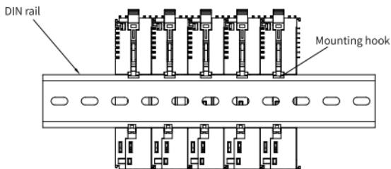
2. Make sure the DIN rail mounting hook of the module is locked. The locked and unlocked states of the mounting hook are shown below.
