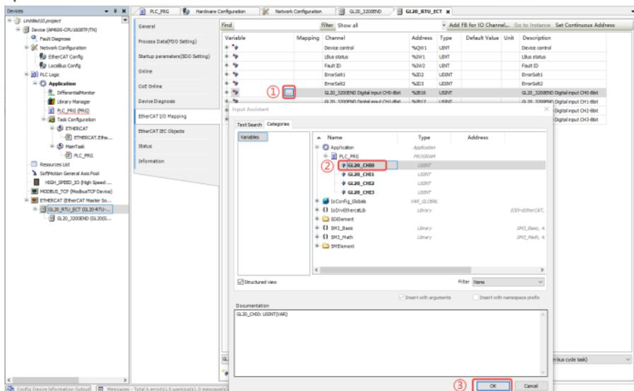
Map the input variables "GL20\_CHI0", "GL20\_CHI1", "GL20\_CHI2", and "GL20\_CHI3" to the input channel of the configuration module, as shown in the figure below.
