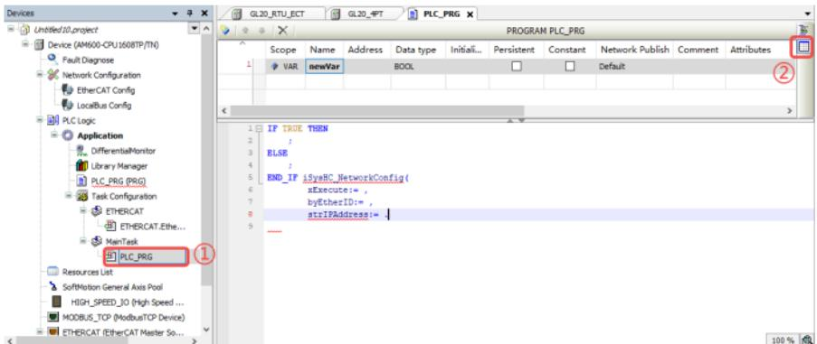
b. Add custom input variables "GL20\_CHI0", "GL20\_CHI1", "GL20\_CHI2", and "GL20\_CHI3". Set the scope of these variables to "VAR" and data type to "USINT", as shown below.
