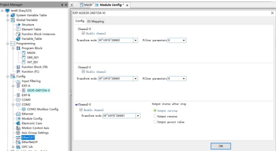
4. (Optional) In the **IO Mapping** tab, you can view the channel mapping elements. The channels are mapped to the system variable "\_ExtCard", as shown in the figure below.
