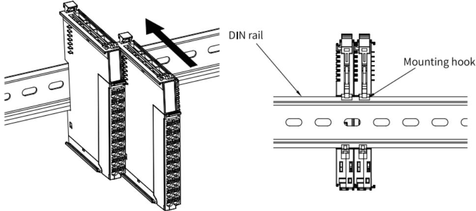
**Note:** After the module is installed, the DIN rail mounting hook will automatically move downward to lock the module to the rail. If the hook does not move downward, press down the top of the hook to ensure that the module is installed in place.
