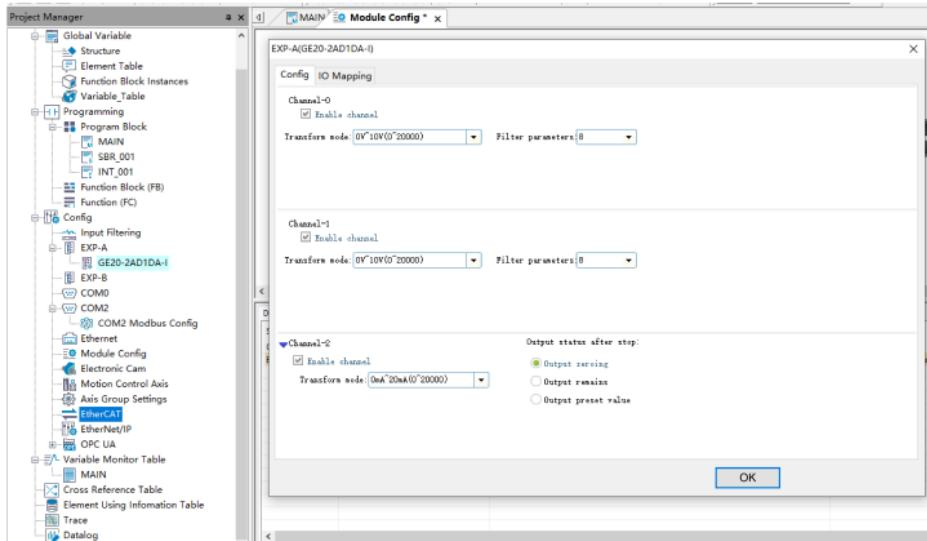
4. (Optional) In the **IO Mapping** tab, you can view the channel mapping elements. The channels are mapped to the system variable "\_ExtCard", as shown in the figure below.
