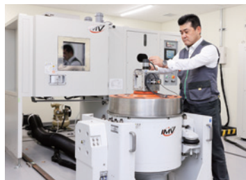
Combined environment testing machine
