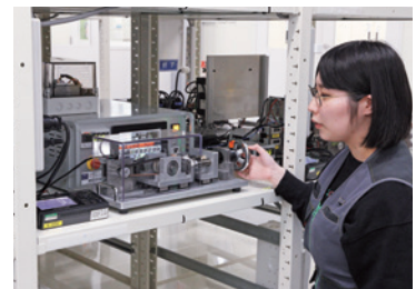
Motor shaft fatigue testing machine
