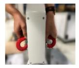
Step 2: Pass the hoisting strap ② through the forearm of the robot and hook the two ends of the strap to the anti-loosening hook of the hoisting strap ①.
