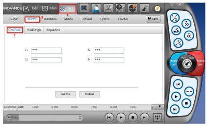
3. Move each joint of the robot to the home position.
