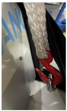
3. Secure the two arms using a strap ①;Pass the strap ② through the forearm of the robot;Attach the other anti-loosening hook of the hoisting sling to the strap ②.
