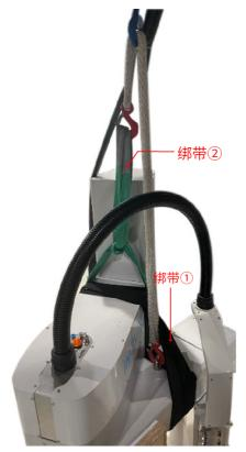
4. Move the robot by two people, with one stabilizing the robot during transportation, and the other operating the crane to lift the robot and move it to the mounting stand.
