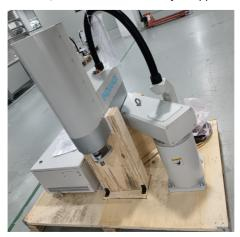
2. Attach one hook of the hoisting sling to the eyebolt on the robot. Ensure the hooking is reliable.
