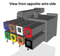
Pin 5 (active low) is a digital stop input, which disables the motor drivers in the icon completely. Pin 6 (active high) is a fault output. Any fault detected is indicated by a change from 0 VDC to 3.3 VDC at this pin. Pin 3 is a signal GND connection.
