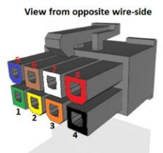
Pin numbers refer to Molex 8-pin connector. Signal GND and Power GND is connected inside the icon.
