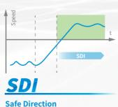
Prevents the motor from rotating in undesignated direction.
