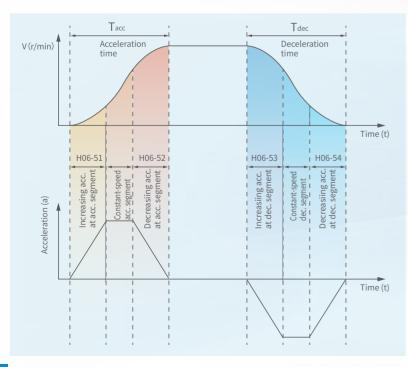
The SV680 series servo drive is supports S-shaped speed curves, allowing users to smoothen the acceleration/deceleration process through controlling the change rate of acceleration/deceleration, without the need for prolonging the motion time. (This function is available in speed control mode only.)
