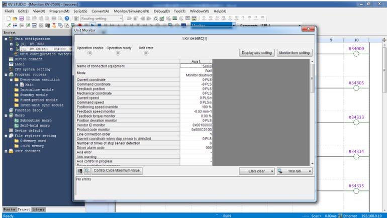
The error state of the unit can also be displayed in the **Unit monitor**. The axis error can be cleared using the **Error clear** button in the bottom right.
