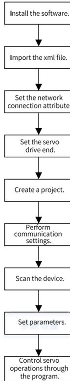
Figure 2-10 Configuration flowchart
