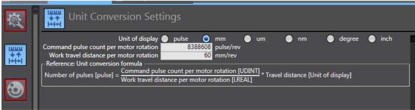
Select **Unit of display** based on the actual operation unit and set the gear ratio. All the position-type parameters in the host controller will be displayed in this unit.
