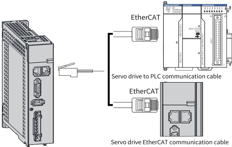
Figure 2-2 Wiring of communication cables
