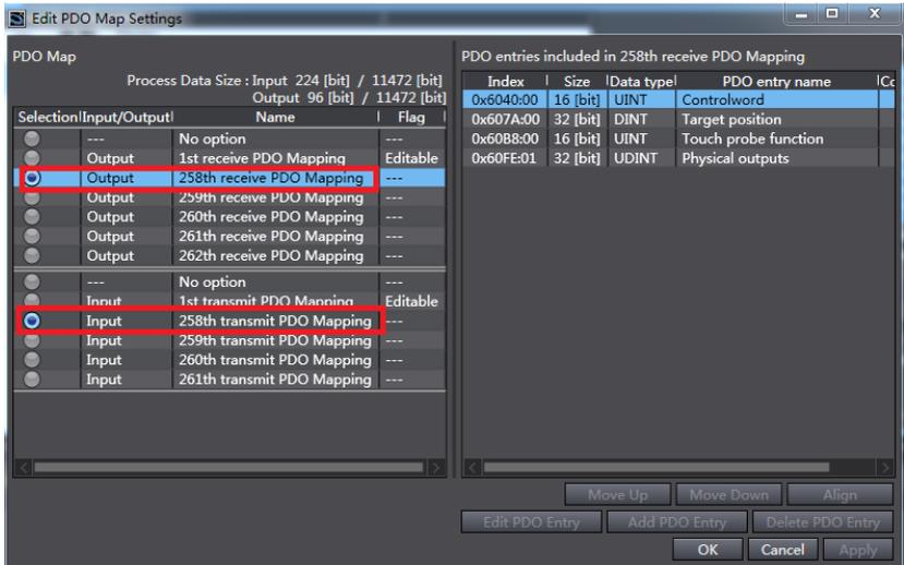
3. Modify the PDO mapping object through **Add PDO Entry** and **Delete PDO Entry**. The commonly used mapping parameters are shown in the following interface.
