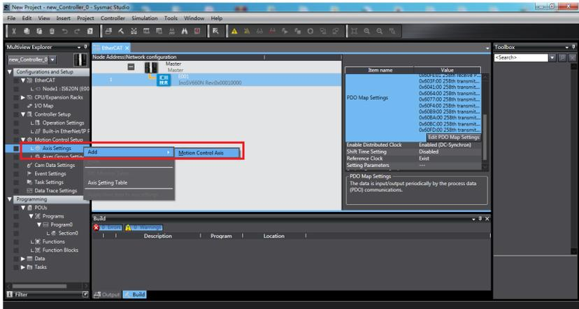
2. MC\_Axis000 can be renamed through a simple click. For example, if it is named as "Rewind axis", the axis variable "Rewind axis" used in the NX program represents control on this SV660N servo axis.
