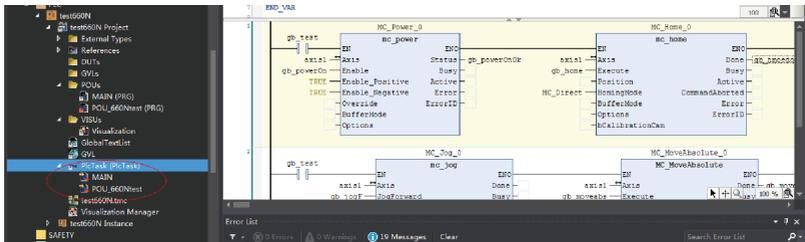
e. Link the axis to the variable defined in the PLC.
