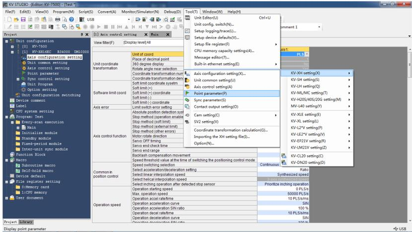
Set the target coordinate and speed per positioning segment as needed. After settings are done, you can call the corresponding **Point No.** through the program to start operation.
