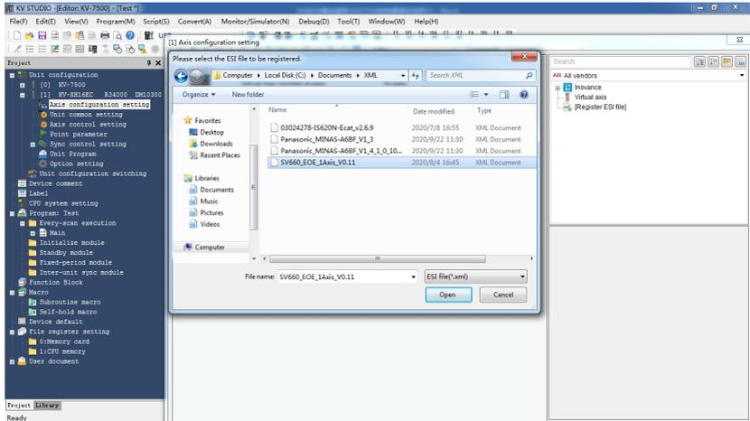
3. After the device description file is imported, you can start to add axes and set the control cycle in **Axis configuration setting**. The default control cycle is 1 ms and the minimum control cycle is 250 us.
