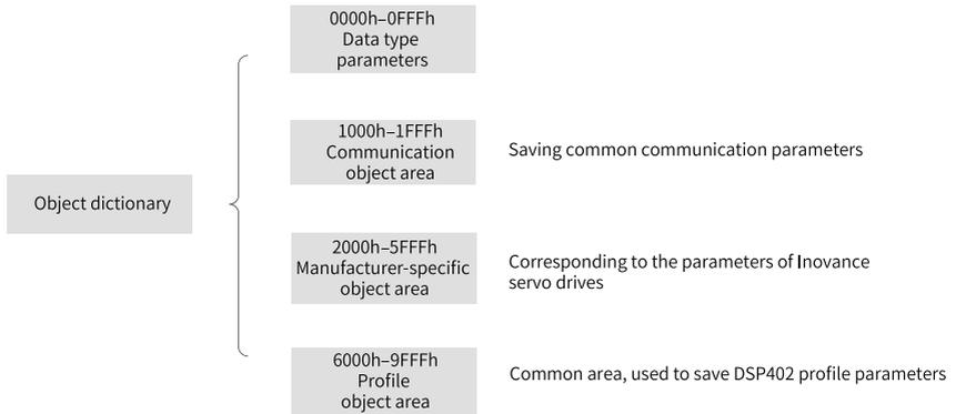
Figure 2-8 Structure of CANopen object dictionary
