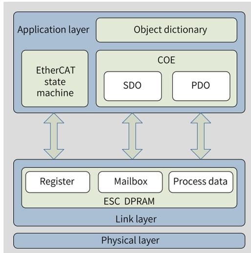
Figure 2-5 EtherCAT communication structure at CANopen application layer
