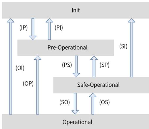
Figure 2-6 EtherCAT state machine
