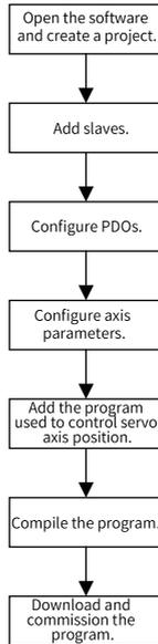
Figure 2-9 Configuration flowchart
