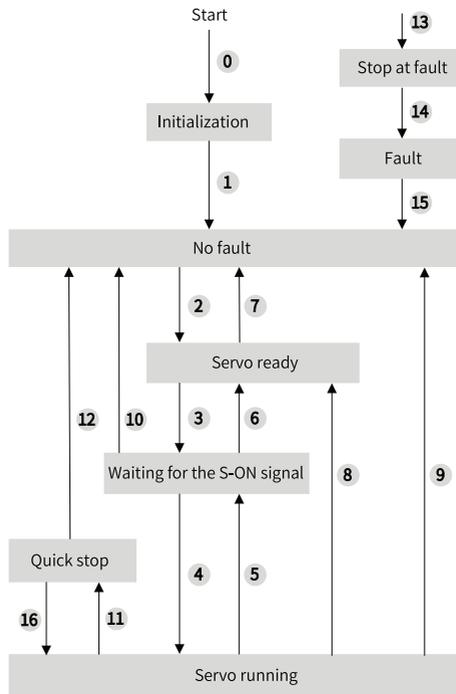
Figure 2-3 CIA402 state machine switchover
