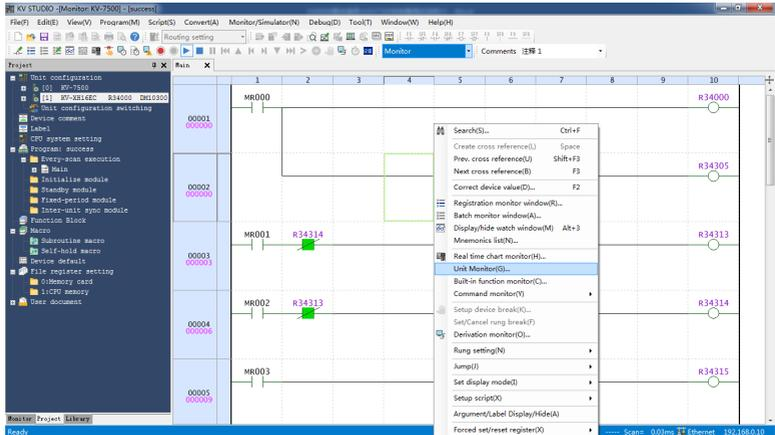
b. The unit monitor displays the operating state of each axis.
