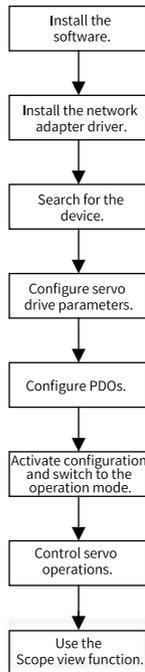
Figure 2-11 Configuration flowchart
