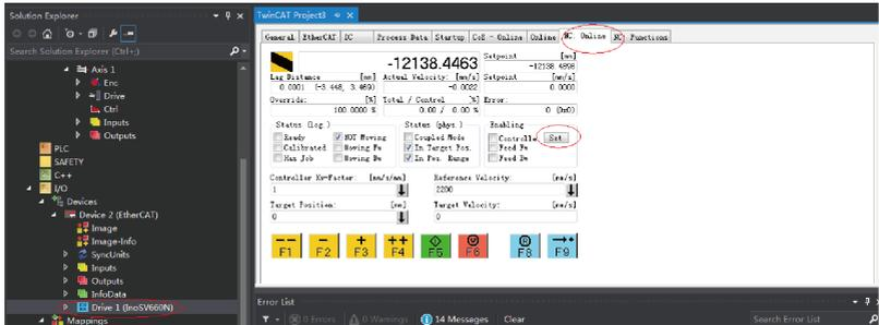
Click **Set** to display a dialog box and then click **All** to enable the servo drive. Perform jogging through F1 to F4. The jog speed is set as follows.
