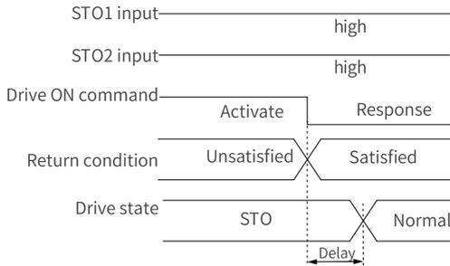
Figure 6-2 Return condition of servo ON/RUN command
