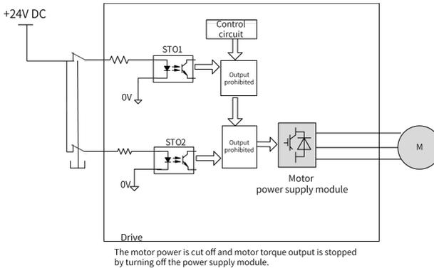
Figure 6-1 Schematics of the STO function
