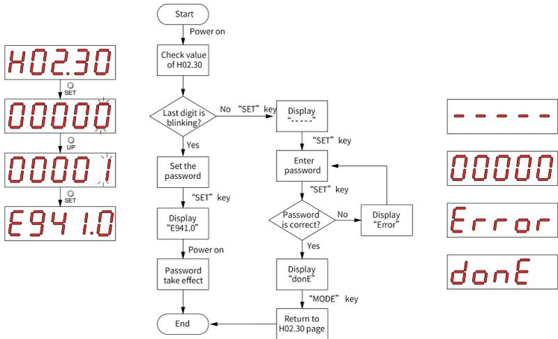
Figure 5-15 Procedure for setting the user password
