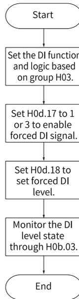
Figure 5-6 Procedure for setting forced DI function
