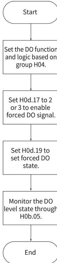
Figure 5-9 Procedure for setting forced DO function
