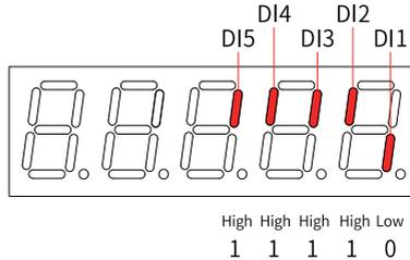
Figure 5-8 DI level status corresponding to H0b.03
