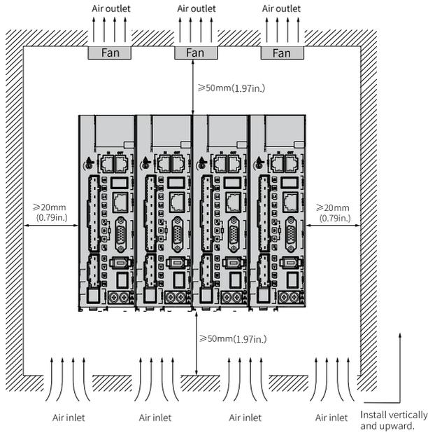
Figure 3-5 Zero-clearance installation
