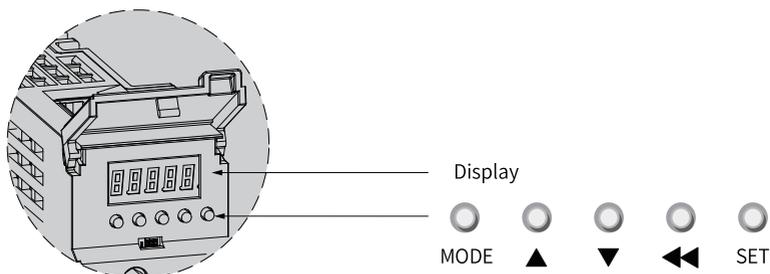
Figure 5-1 Magnified view of the operating panel
