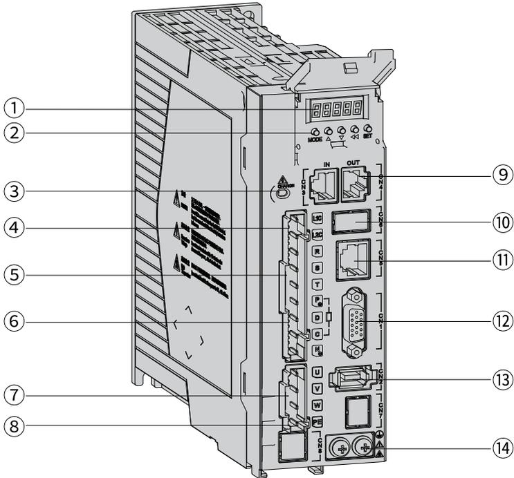
Figure 2-4 Components of servo drives in size C (SV660NT3R5I and SV660NT5R4I) and size D (SV660NT8R4I and SV660NT012I)
