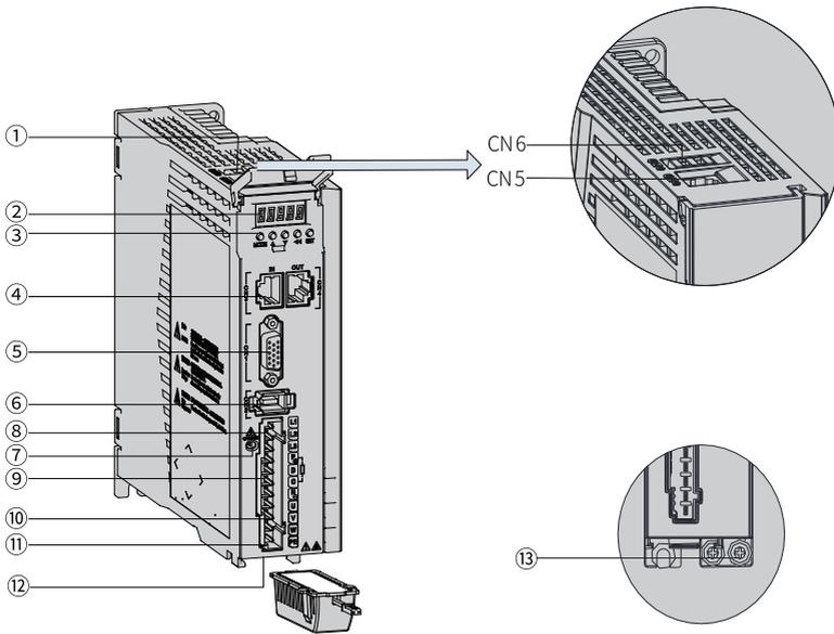
Figure 2-2 Components of servo drives in size B (SV660NS5R5I)
