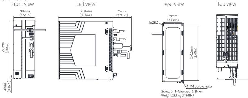
Figure 3-10 Outline dimensions of servo drives in size E
